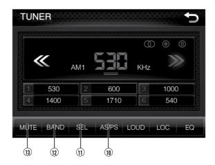
Automatically Store / Preset Scan (10) Press and hold **AS/PS** to automatically find and store the strongest stations as presets. Press **AS/PS** momentarily to scan preset stations and play 10 seconds of each.
